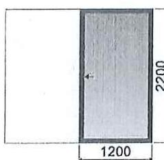
Coulissant Aluminium LALOI Menuiseries Gamme CL32 Rupture thermique totale Finesse chicanes 35mm Classement A4 E9b VC2\*
